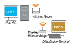
Take the benefit of OfficeStation Solution to the next level by adding wireless protocol. \*802.11g Wireless router and bridge required
