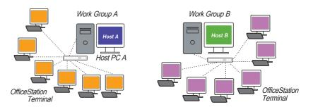
Great saving on hardware cost as well as IT maintenance when OfficeStation network terminal solution is implemented. Multiple host PCs can be connected under the same corporate network environment for department/group computing.
